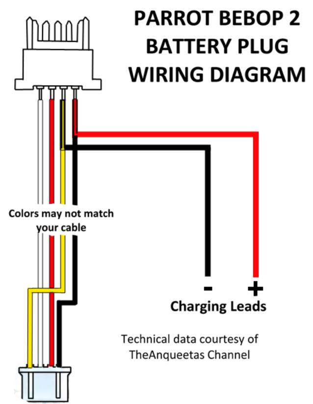
To balancing socket of charger Guide tabs shown "up"
